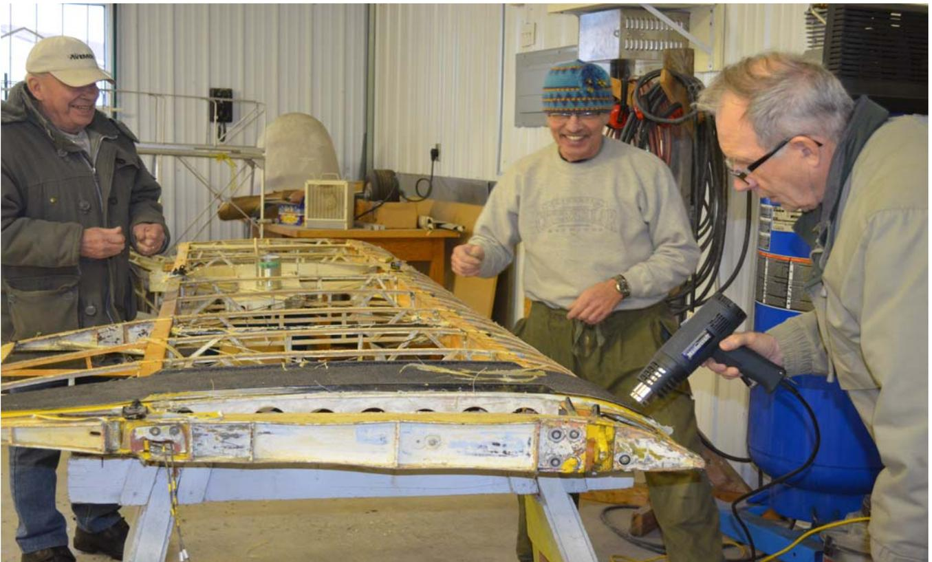
*Vic Prefontaine and Rick Riewe look on as Ken Podaima tries out using a heat gun to loosen the packing tape stuck to all the surfaces*
