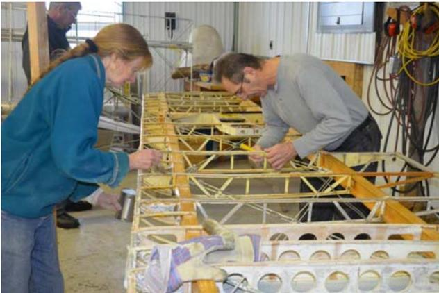
*Jill Oakes and Gilbert Bourrier stripped five layers of paint off the ribs so they could be inspected for wood rot and fractures. Approximately six broken or split ribs were found and are currently being repaired.*
