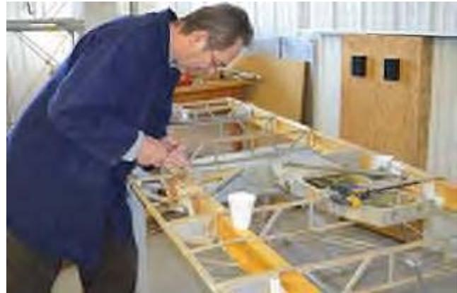
*Gil Bourrier prepares the surface for gluing on a newly fitted cap strip from Bill LeBrun's donation of sitka spruce - for the nose rib near the aileron control box.*
