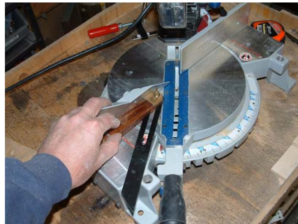
Figure 3: Transferring Angle to the Saw
