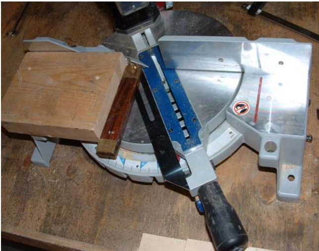
Figure 4: Transfer Bevel Angle to Saw
