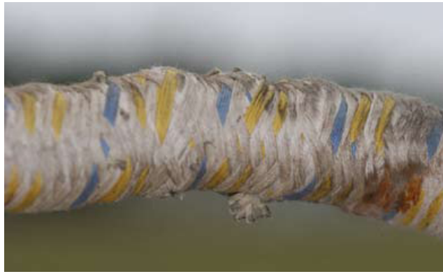
This cord shows obvious signs of damage to the outer covering and the rubber strands inside. The bumps and breaks in the covering indicate many broken strands inside the shock cord. This cord must be replaced.
