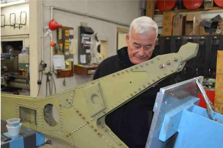
*Blackner checking out the engine mount made by TSA For the Mustang*
