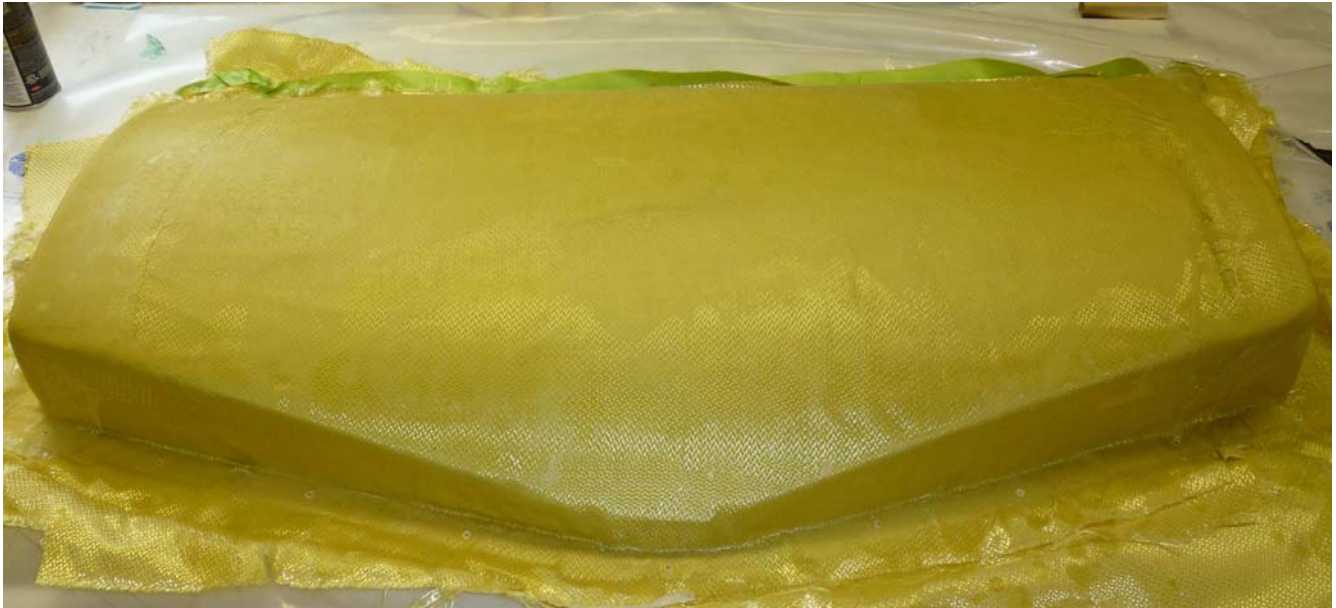
Illustration 3. Fuel Tank Vacuum Formed Using Kevlar Cloth
