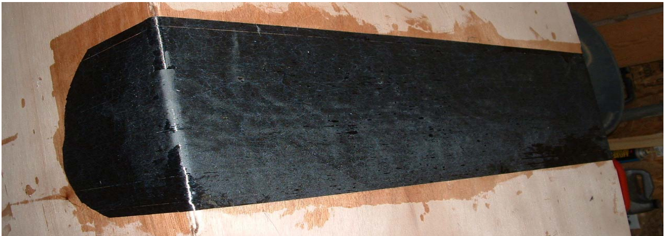
Illustration 1: Unidirectional Carbon Fiber Applied to Strengthen a Fuselage
