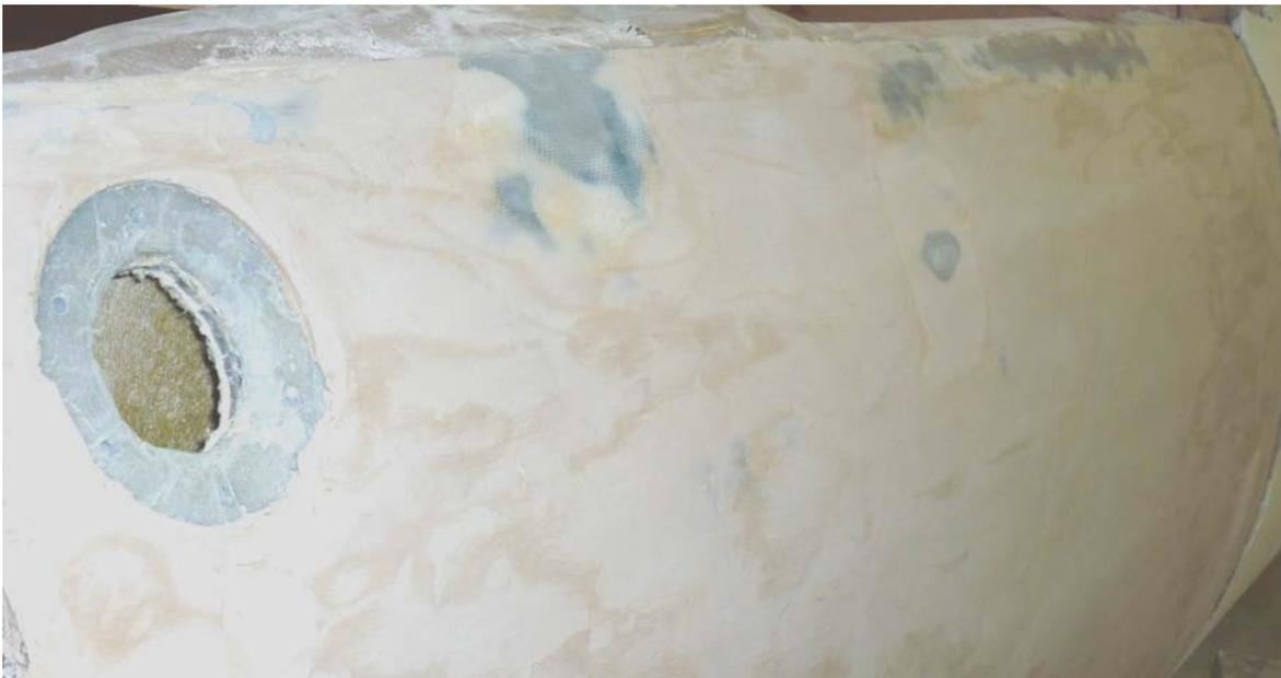
*Figure 2: Finished Composite Surface (Almost) Ready for Painting*
